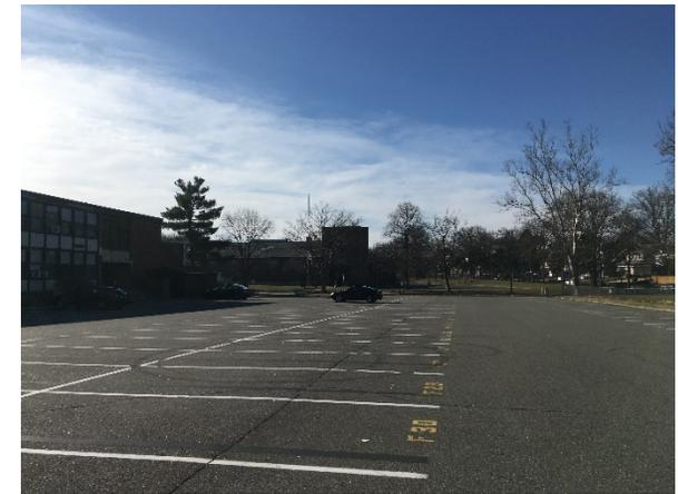
A rain garden can be installed on the island adjacent to the south of the parking lot to capture, treat, and infiltrate stormwater runoff from the lot. Additionally, pervious pavement can be installed in parking spaces to capture and infiltrate parking lot runoff. A preliminary soil assessment suggests that more soil testing would be required before determining the soil's suitability for green infrastructure.
