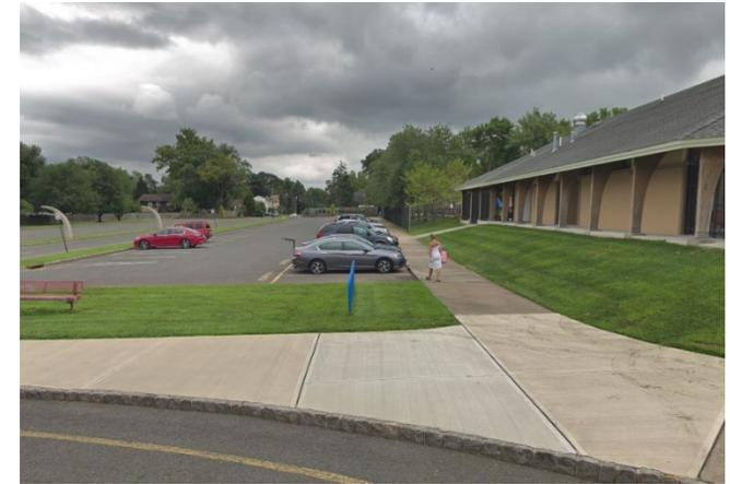
Large rain gardens can be installed in the turfgrass island dividers of the parking lots. A smaller rain garden can be installed adjacent to the building to manage stormwater runoff from the rooftop. Additionally, pervious pavement can be installed in a section of parking spaces to capture the remaining stormwater runoff from the surrounding asphalt. A preliminary soil assessment suggests that more soil testing would be required before determining the soil's suitability for green infrastructure.
